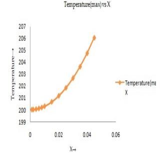
Fig-3 Variation of temperature of triangular fin with length  $\left( L\right)$
