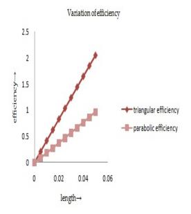
Fig-6 Variation of efficiency( $\eta)$  of fin with length of fin(L)
