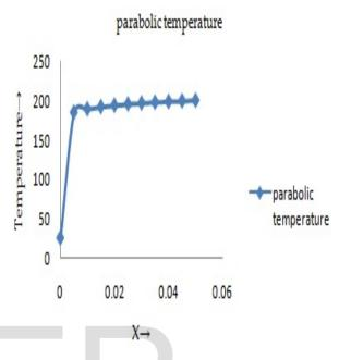
Fig-4 Variation of temperature of parabolic fin with length(L)  $% \left( {{{\rm{D}}_{{\rm{A}}}}} \right)$
